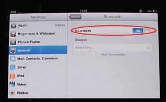
Step 3: The keyboard will search the Bluetooth devices automatically after turning on the Bluetooth function. Once you've found "Bluetooth mini Keyboard", chose this device and it will start connecting with a pass word displayed.
